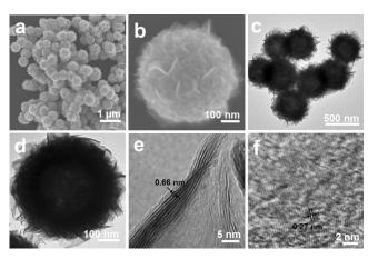
**Figure 3.** a),b) FESEM and c),d) TEM images of the  $MoS_2$  HNS after annealing in  $Ar/H_2$  at 700°C for 2 h. e),f) HRTEM images of the  $MoS_2$  sheets
