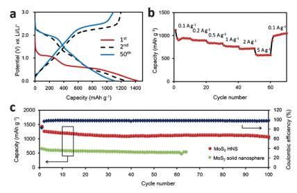
**Figure 4.** a) Charge–discharge voltage profiles at  $0.5 \, \text{Ag}^{-1}$ , b) rate capability test, and c) cycling performance at  $0.5 \, \text{Ag}^{-1}$  of the  $\text{MoS}_2$  HNS and of  $\text{MoS}_2$ . The blues trace shows Coulombic efficiency of  $\text{MoS}_3$ , HNS.
